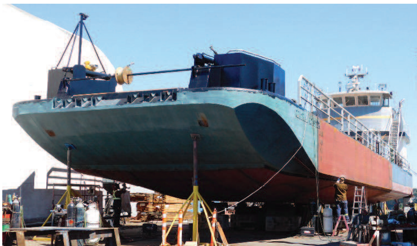
LEFT The Central Coaster's new 60-foot double-hulled midsection was fabricated by Canron Western Constructors in Delta, and welded in place between the refitted original bow and the new 30-ft extension at the stern.
