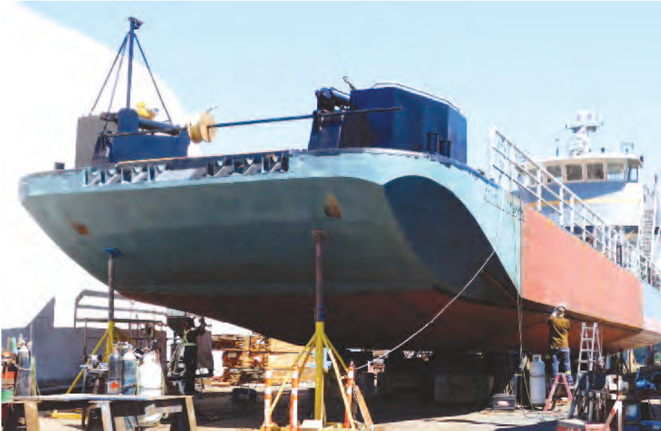
The Central Coaster's new 60-foot double-hulled midsection was fabricated by Cannon Western Constructors in Delta, and welded in place between the refitted original bow and the new 30-ft extension at the stern.
